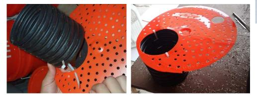
**Step 3**— Place the other 2 (8 ring long) drain pipes in the base of the bucket. Put the plastic divider with attached pipe inside the bucket so that all three pipes fit next to each other. Hold the bucket up to the light so you can locate the point on the side of the bucket that is just at or below the plastic divider. Drill a hole using the 3/8" drill bit for over-flow drainage. If you are using Home Depot buckets,
